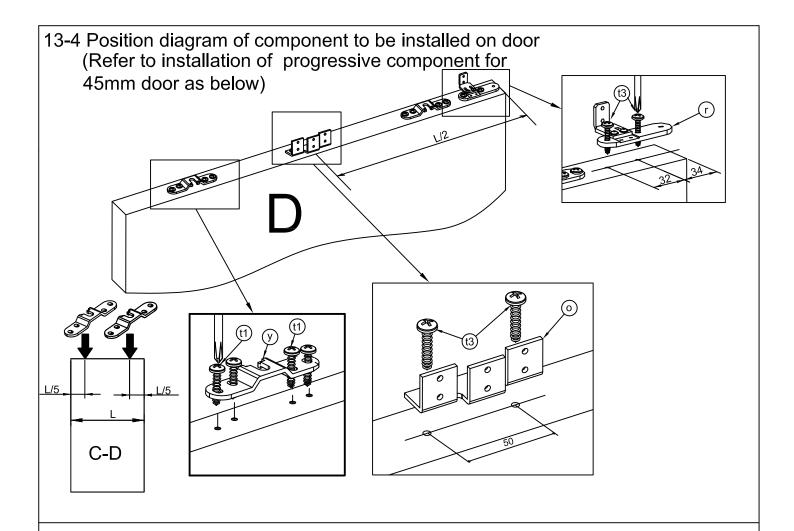
Note: component "r" has also an adjustable bending plate "rr"on it, for different door thickness, position of "rr" can be adjusted to meet installation requirement. Different installation diagram as below:
